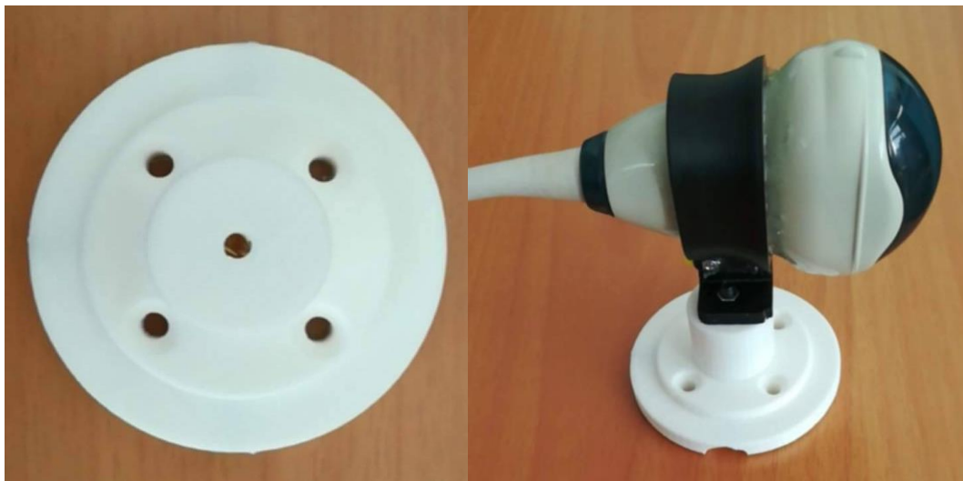
Figure 22 - Picture of the 3D printed holder and its assembly to the US probe hoop (on the right).
