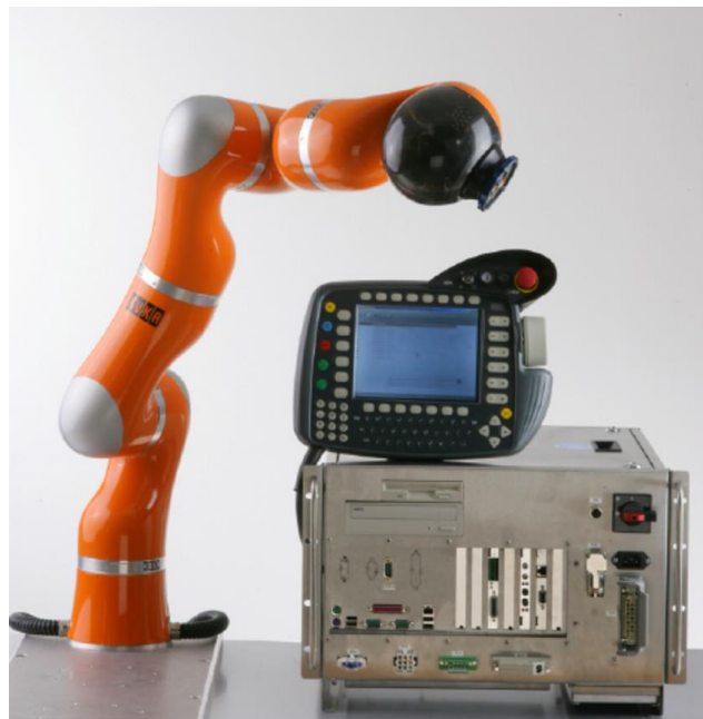
Figure 18 - KUKA LWR with controller and KUKA control panel (KCP.) [70]
