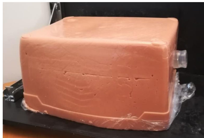
Figure 13 – Picture of the final liver phantom.
