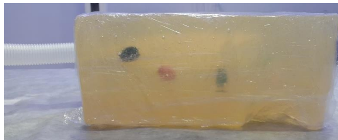
Figure 10 - First phantom developed with a homemade echogenic medium.
