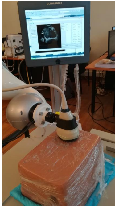
Figure 32 - 3D US Image acquisition of the liver phantom using the US-Robot setup.
